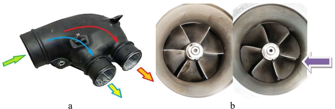
Fig.7. Branch pipe for the flow from the air filter to the turbochargers of the right and left rows of cylinders of a V-8 engine (a) and the inlet edges of the turbocharger blades [4] as a result of operation over 42,000 km of vehicle mileage (b).
